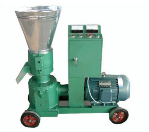
**Figure 3.** Flat-die pellet mill machine.
