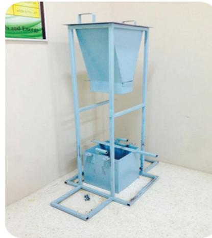
**Figure 4.** Testing machine for bulk density.
