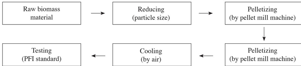
**Figure 2.** Production process of sugarcane bagasse and eucalyptus bark pellets.
