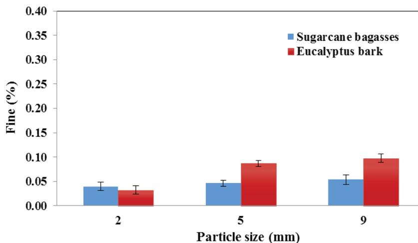
Figure 8. Effect of particle size on pellet fines content of bagasse and eucalyptus bark.
