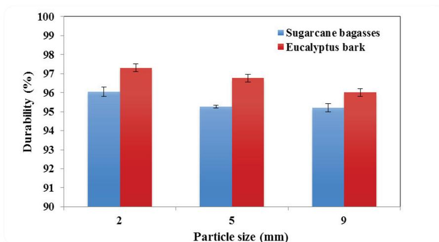
Figure 7. Effect of particle size on durability of bagasse and eucalyptus bark pellets.
