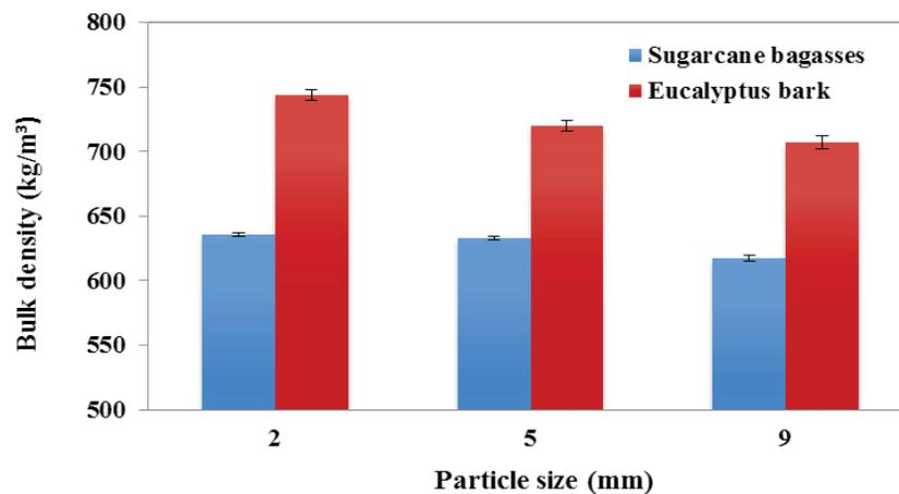
Figure 6. Effect of particle size on bulk density of bagasse and eucalyptus bark pellets.
