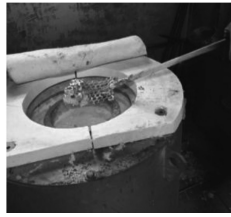
Fig.1 melting at 720 °C with induction furnace.
